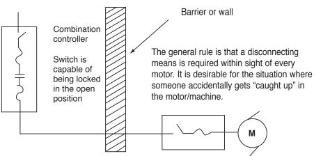
Figure 9: Use of Motor Disconnecting Means
