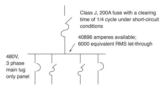
Figure 3: Circuit using Current-Limiting Fuses
