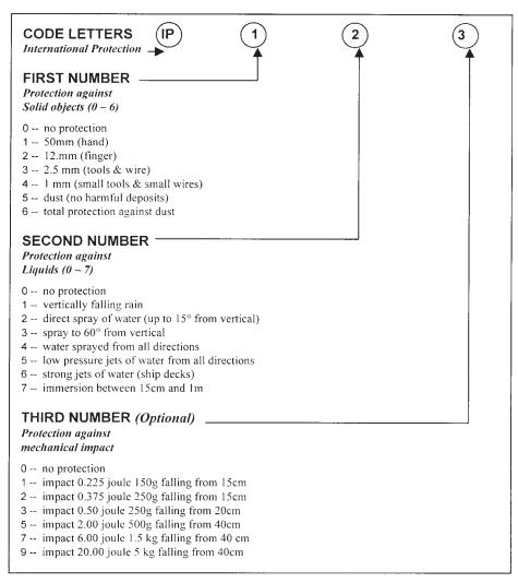
Figure 6. IP Environmental Ratings for Enclosures (IEC 529)
