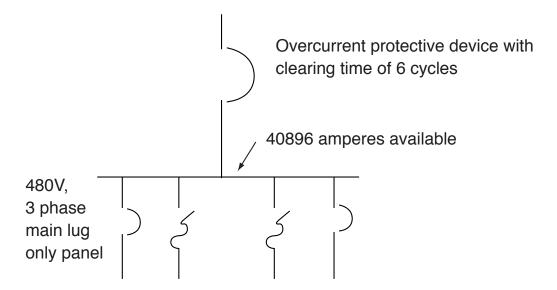
Figure 2: Circuit using Non-current Limiting Circuit Breakers
