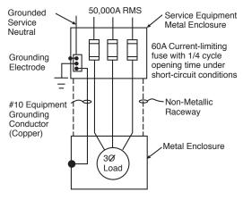
Figure 8: Complies with NEC Section 110.10 and 250.4(A)(5)
