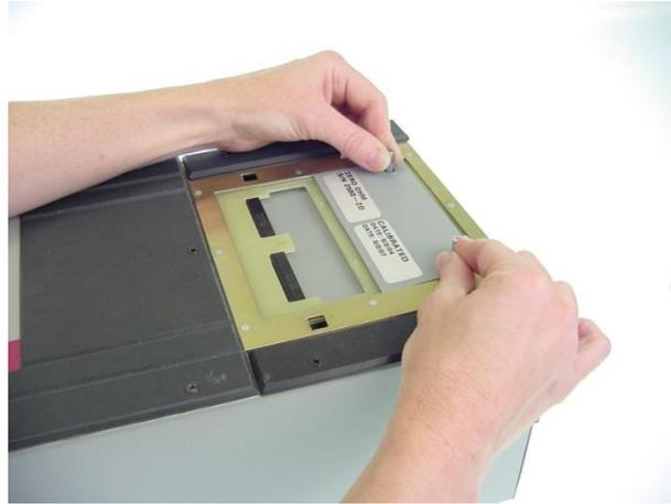
6. If the tester has any expansion boxes installed, continue testing the other scanners by moving the Zero Ohm Adapter to each of the "J" positions and running the test.
