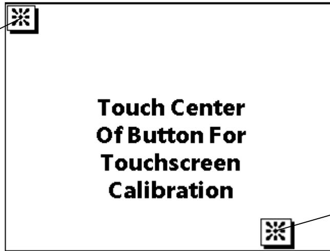
**Step 2:** Use a pointed object to touch the center of the button.
