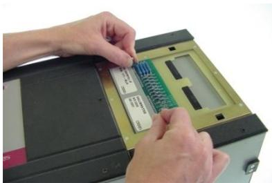
4. Touch the tip of the probe to the exposed pads of any test points on the adapter. If the probe is working correctly, a pop-up window will display the correct point(s) touched by the probe. If no pop-up window is displayed when the test point(s) are probed, press **No Response.** The test will fail and a Failed Probe Test screen will display.
