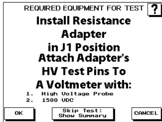
A high voltage probe is required to perform the HV Volts test.
