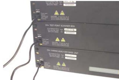
2. The serial cable is connected from the serial port of the computer to the serial port on the base unit of the tester.
