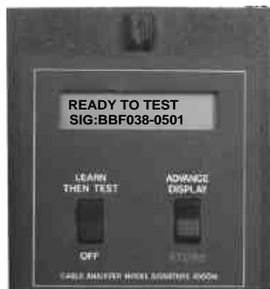
Cable retrieved, adapters are correct. You are ready to test.
