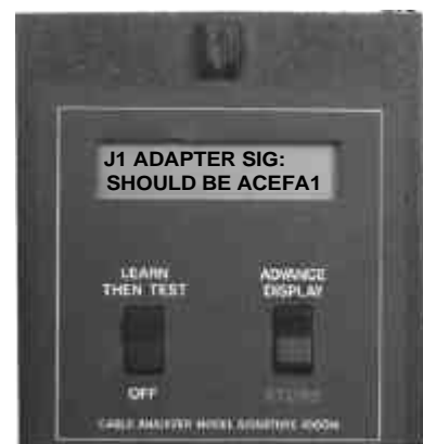
Installed adapters are not correct. Install correct adapters. When you've done that, prompt will change to Ready to Test .
