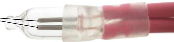
**Note:** If the lamp electrodes were surrounded by air, a hipot voltage over 5000 volts would be required to cause an arc. However, the neon gas inside the lamp breaks down at a much lower voltage than air; therefore, a 500 volt test creates arcing.
