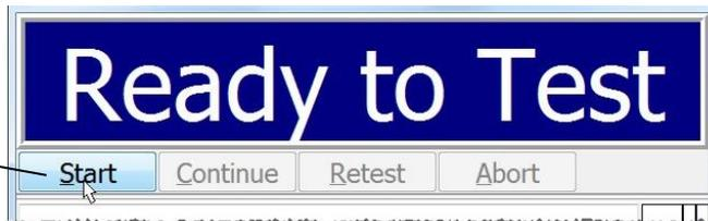
The tester will perform a low voltage test. If it passes, the display changes to “Ready to Hipot.”
