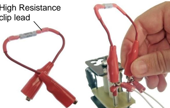
**Note:** The “high resistance clip lead” has a 90 MOhm resistor that simulates an Insulation Resistance (IR) failure. The Insulation Resistance test verifies that the resistance offered by the insulating materials is sufficiently high. Failure occurs when the measured resistance value is lower than the specified value. In the demo, our IR setting is 150 MOhms; therefore, the 90 MOhm resistor is seen as an IR Leakage failure.
