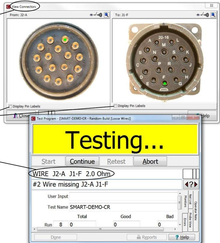
LEDs blink green to show the connectors of the from/to test instruction.
