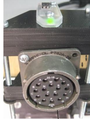
The green dots in the connector image indicate the cavity for the missing wire.
