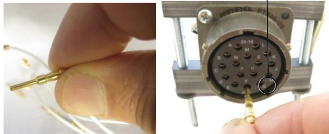
**Note:** Once the pin is inserted in the correct position the inserted pin location turns blue, and the "from-to" pins locations for the next test instruction are displayed in green. In this example the inserted pin was J1-F.
