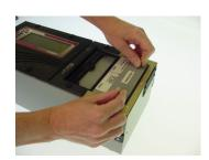
14. If you installed add-on scanners, move the Zero Ohm Adapter to each subsequent "J" position and repeat steps 2-9 for each test.
