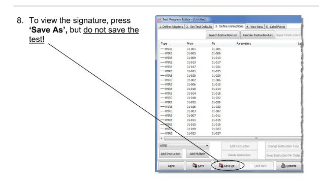
If the displayed signature matches the correct signature on the verification data sheet under "Signal Routing System Test", check off Pass; otherwise, check off Fail.
