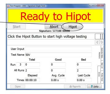
Record the voltmeter value on the verification data sheet under "HV System Test, 50 Volt." If the voltmeter value is between the minimum and maximum limits shown in Table 3, check off Pass; otherwise, check off Fail.
