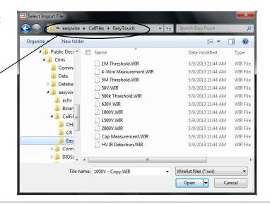
5. Press the "Name" check box to select all of the verification files as shown, and press 'Open'.
