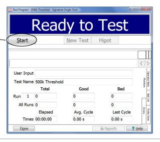
4. The test window should display "HIGH RESISTENCE ERROR". If the failed points are from J1B016 to J1A016, check off Pass on the verification sheet under "Resistance Threshold System Test,  $500k\ \Omega$ "; otherwise check off Fail.
