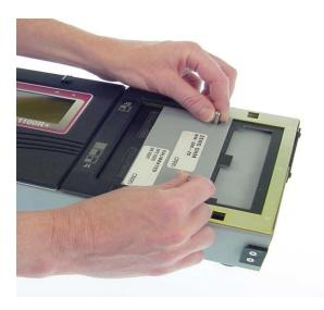
3. Press the BACK button and then press **LEARN.** The tester will learn the cable and display the CABLE LEARNED screen. The screen will display TEST:7F5527-6M020 where 7F5527-6M020 is the cable signature. Write the signature you see on the verification sheet. Compare it with the Correct Signature shown on the sheet and check off either Pass or Fail.
