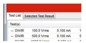
The details of the specific test as well as the measured values will be displayed.
