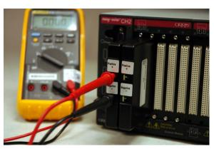
7. Read the meter and enter the value (in volts) into the box on the Verification Assistant and click **Okay.**
