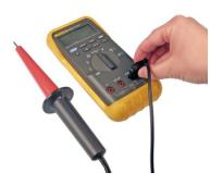
3. Connect your high voltage probe to the test pins on the Resistor Leak adapter as shown.
