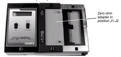
2. Turn on the analyzer. The analyzer will prompt Learning Cable for several seconds, then the prompt should change to SIG:XXXXXX-XXXX Please Verify. The correct signature will be shown on the data sheets. Write the displayed signature into the "Signature Seen" blank in Table 1 on the data sheet, then compare it to the "Correct Signature" shown. If they match, check off "Pass." If they do not match, check off "Fail".
