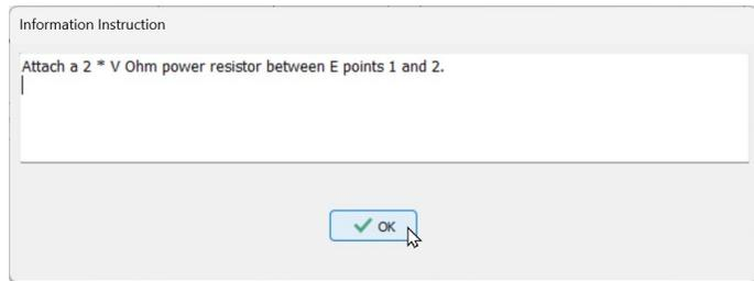
5. Use the voltmeter to measure the voltage between Energization (E) points 1 and 2. If the voltage is less than 10mV, click **Yes**, otherwise click **No**.
