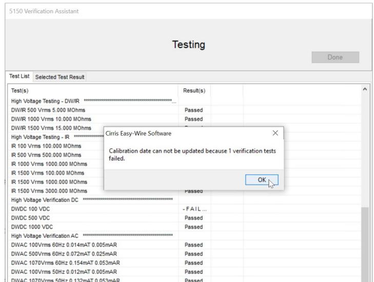
If the meter measurements were entered correctly, a failed result indicates that the Base Unit requires service.
