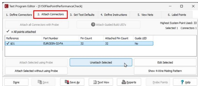
4. With the connector still highlighted, click **Attach Selected without using Probe**.
