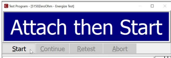
3. Follow the instructions in the pop-up window and install the Zero Ohm Adapter on Scanner Module 1. Scanner Module 1 is the left most scanner in the Base. (See note on next page regarding Flex Modules).
