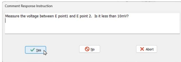
6. Use the voltmeter to measure the voltage between the same two points. If the voltage is within 2.5V of the Energization supply, click **Yes**, otherwise click **No**.
