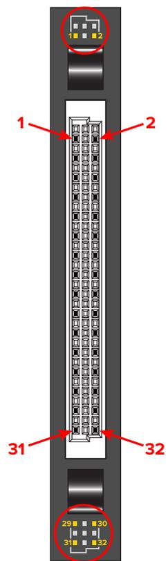
4. When the first instruction is displayed, attach the power resistor that has an ohm value equal to two times the Energization voltage between Energization (E)points 1 and 2. Click **OK**
