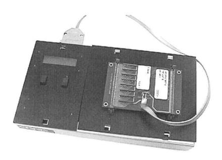
Test adapter installed with J1 on adapter plugged into J1 on analyzer. Note that the row of SIP resistors on the adapter is close to the analyzer's LCD display
