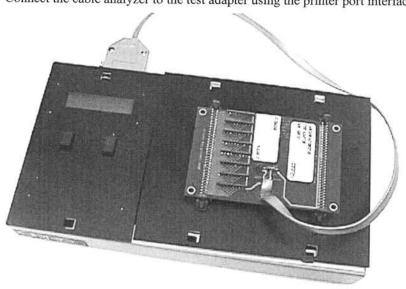
Test adapter connected to analyzer using printer port interface
