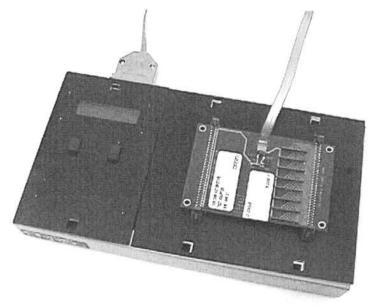
Test adapter installed with J1 on adapter plugged into J2 on analyzer. Note that the row of SIP resistors on the adapter is oriented to be as far as possible away from the analyzer's LCD display.
