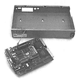
3. Pop out the plastic covers from the rectangular openings in the sides of both boxes (if they're there), snake the long ribbon cable through the rectangular openings in the sides of both boxes. (**Note**: If you can't see the long ribbon cable, it's stowed inside the alarm box. Remove the quarter-turn fasteners, lift out the top assembly, and feed the ribbon cable through the opening in the side
