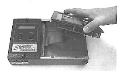
In this view, the quarter-turn fasteners which hold the scanner assembly on the analyzer have been opened, and the cover plate has been removed. The scanner assembly has been lifted from the chassis. Note that the ribbon cable which connects the scanner with the rest of the analyzer is still connected.
