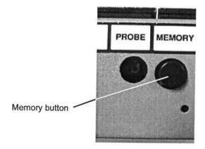
3. The analyzer will prompt SIG:XXXXXX-XXXX Please Verify. Be sure to use the correct data sheet for the firmware version your analyzer has. Write the displayed signature into the Signature Seen blank in Table 10 on the data sheet. Compare the signature prompted by the analyzer with the Correct Signature. If they match, check off "Pass." If they do not match, check off "Fail."
