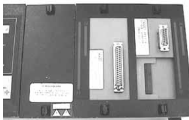
Double-high adapter in J1-J2, single-high adapter in J4
