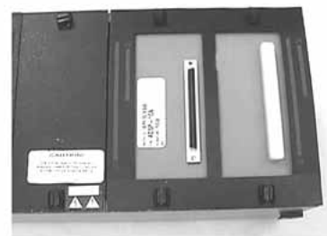
Quad-high adapter mounted in scanner positions J1, J2, J3, J4
