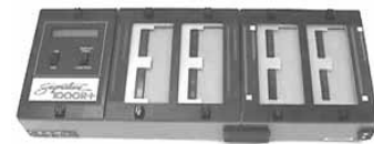
1000R+ with 1 expansion box installed. Eight "J" positions (256 test points) are available.
