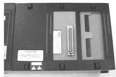
Double-high adapter mounted in scanner positions J1, J2
