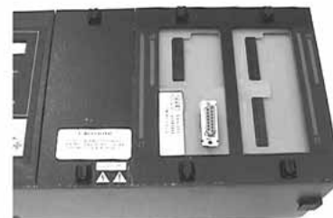
Single-high adapter mounted in scanner position J1.
