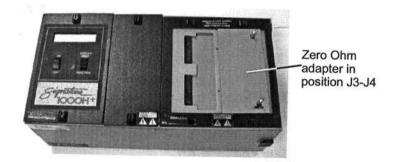
4. Turn on the analyzer. The analyzer will prompt Learning Cable for several seconds, then the prompt should change to SIG:94C424-6N030 Please Verify. Write the signature you see into appropriate table on the data sheet, compare it with the Correct Signature shown in the table, and check off either Pass or Fail. Turn off the analyzer.
