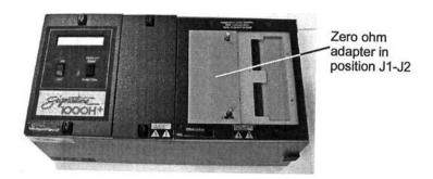
2. Turn on the analyzer. The analyzer will prompt Learning Cable for several seconds, then the prompt should change to SIG:7F5527-6N030 Please Verify. Write the signature you see into appropriate table on the data sheet, compare it with the Correct Signature shown in the table, and check off either Pass or Fail. Turn off the analyzer.
