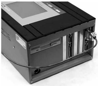
Plug adapter into Digital I/O port
