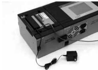
Plug DC power adapter into SCSI testing adapter
