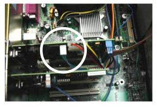
Locate the Three Pin Tiny connector.
