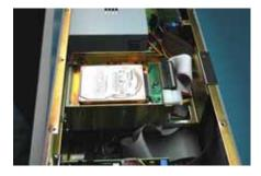
Place the Floppy/Hard drive cage into the chassis.
