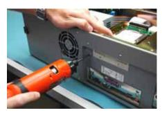
Align the holes on the cage with the holes on the chassis.
