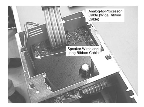
11. Connect the long ribbon cable, and the wide Analog-to-Processor ribbon cable to the connectors on the processor as shown here.
