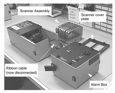
In this view, the Scanner Assembly has been disconnected, and set aside lying on its top. The Scanner Cover Plate has also been set aside.
