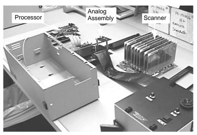
In this view, the Processor Assembly and the Scanner Assembly have both been laid aside lying on their tops. The analog assembly with its metal frame has been lifted out of the chassis, and set on the bench.
