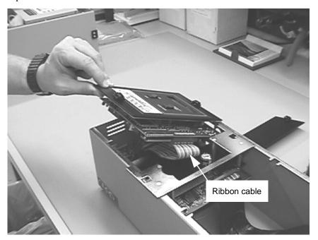
5. Turn the Processor Assembly over gently. You'll see the ribbon cable still connected to it. The wires running to the system speaker are also still connected.
