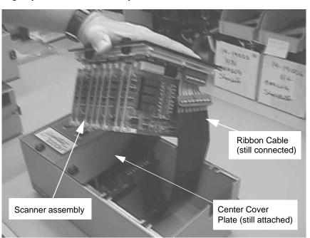
In this view, the quarter-turn fasteners which hold the scanner assembly on the analyzer have been opened, and the cover plate has been removed. The scanner assembly has been lifted from the chassis. Note that the ribbon cable which connects the scanner with the rest of the analyzer is still connected. The center cover plate is still in place on the analyzer's chassis.
