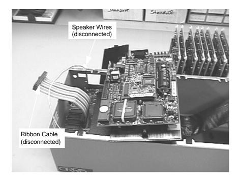
7. Gently, lift the analog assembly up and out of the chassis. The chassis will now be essentially empty.
