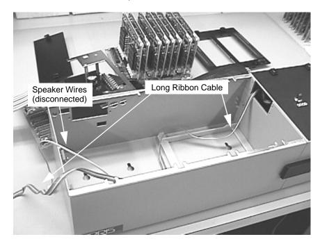
10. Replace the analog assembly (with its metal frame) in the analyzer's chassis. Note that the speaker wires and the long ribbon cable still aren't connected. In the lower photo (with the analog assembly in place), note how the long ribbon cable and the speaker wires run down alongside the analog assembly.
