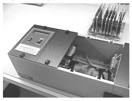
15. Reconnect the Processor-to-Scanner ribbon cable, then lower the scanner assembly carefully back into the chassis as shown here.
