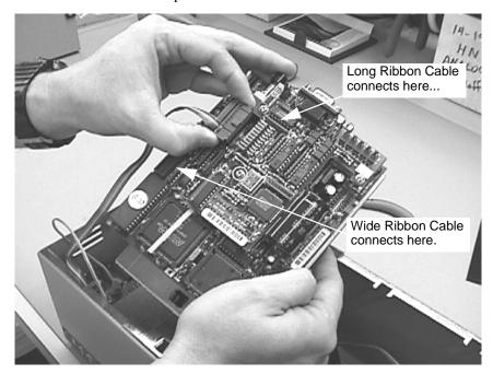
12. Connect the speaker wire as shown here. By now, all three cables (the wide Analog-to-Processor ribbon cable, the narrower long ribbon cable, and the speaker wires should all be connected to the processor assembly. If they're not all connected as shown in this photo, connect them.
