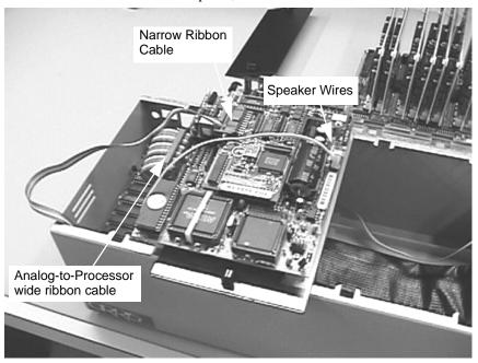
13. With all three cables reconnected to the processor assembly, turn the processor assembly right side up, and carefully lower it back into the chassis as shown here. **Be sure to lower the assembly at an angle as shown!** This will avoid snapping the pogo pin that grounds the processor to the chassis.
