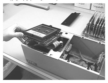
14. Replace the center cover plate as shown here.
