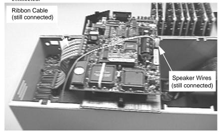
6. Disconnect both the ribbon cable and the speaker wires, and lay them carefully aside. The Processor Assembly is now disconnected from the rest of the analyzer.
