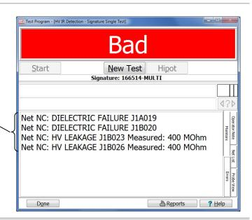
**Note:** The actual measured value for the error will vary on each tester.
