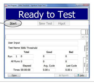
4. The test window should display "HIGH RESISTENCE ERROR". If the failed points are from J1B016 to J1A016, check off Pass on the verification sheet under "Resistance Threshold System Test,  $500k\ \Omega$ "; otherwise check off Fail.
