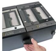
**Note:** Before performing any of the tests in this manual, remove all adapters from the tester (including from the add-on boxes) except for the adapters needed for verification. Failing to remove unnecessary adapters could result in the wrong signature and cause a failure even when the tester is functioning correctly.
