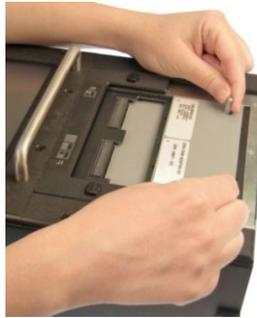
14. If you installed add-on scanners, move the Zero Ohm Adapter to each subsequent "J" position and repeat steps 2-12 for each test.
