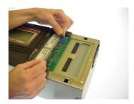
2. Connect your voltmeter probes to the test pins on the Resistor Leak adapter as shown.
